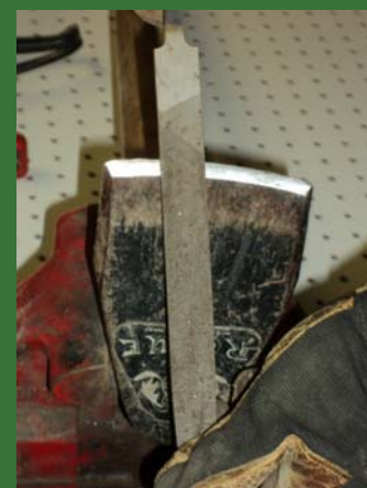
Sharpening the head of a hoe with a file
