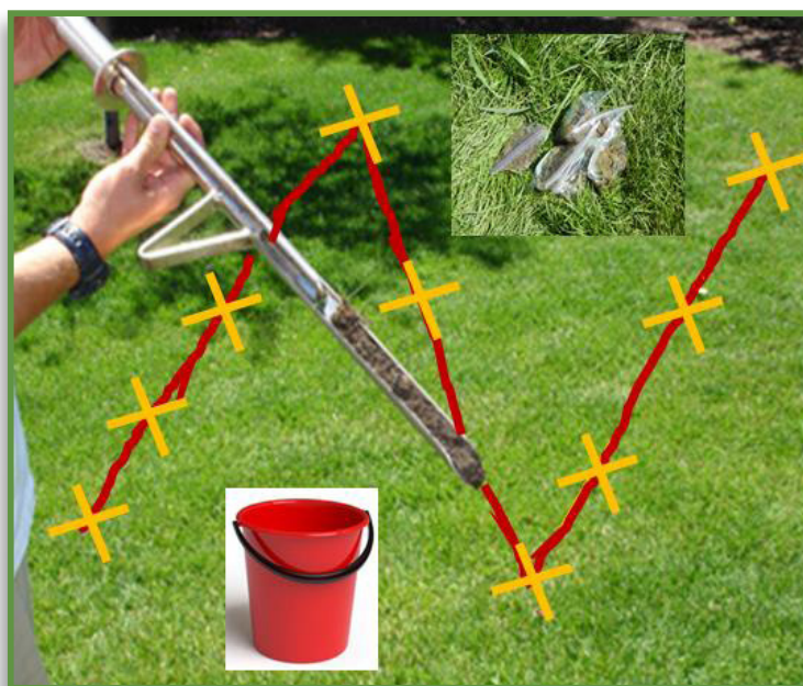
Photo 2: How to take a soil sample: Take 12 cores of soil by zigzagging to cover as much of the sampling area as possible.
