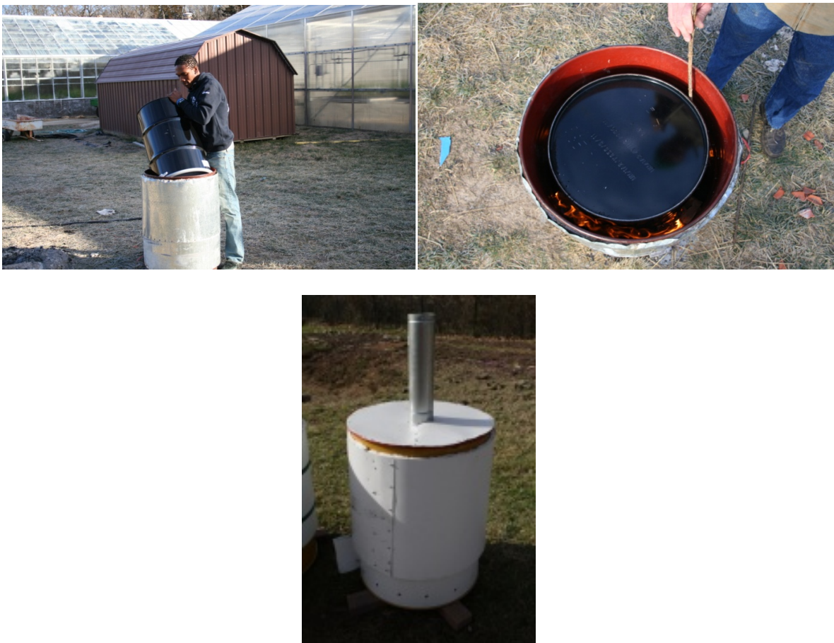
Figure 6. The inner drum fits inside the outer barrel leaving enough space for the initial woody fuel.
