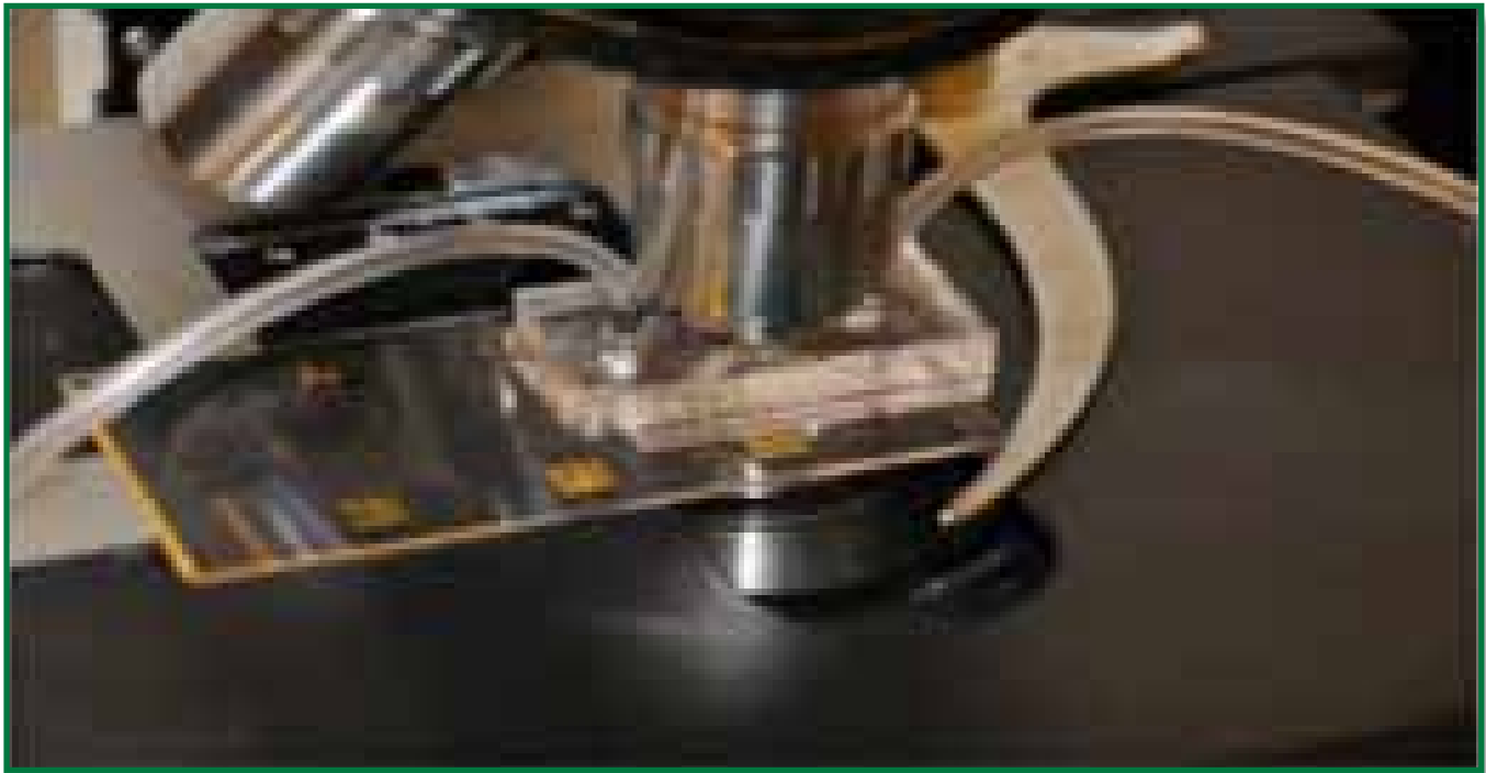
Here is the fabricated biosensor. There are tygon tubes connected to the inlet and outlet.
