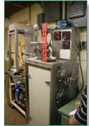
The left image shows the device used for super critical CO 2 extraction at the National Center for Agricultural Utilization Research Center in Peoria, Illinois, as a collaborative effort with Lincoln University. The right image shows a cylinder containing plant materials inside the extraction chamber.
