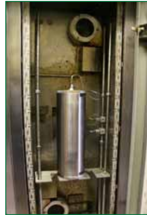
The left image shows the device used for super critical CO 2 extraction at the National Center for Agricultural Utilization Research Center in Peoria, Illinois, as a collaborative effort with Lincoln University. The right image shows a cylinder containing plant materials inside the extraction chamber.
