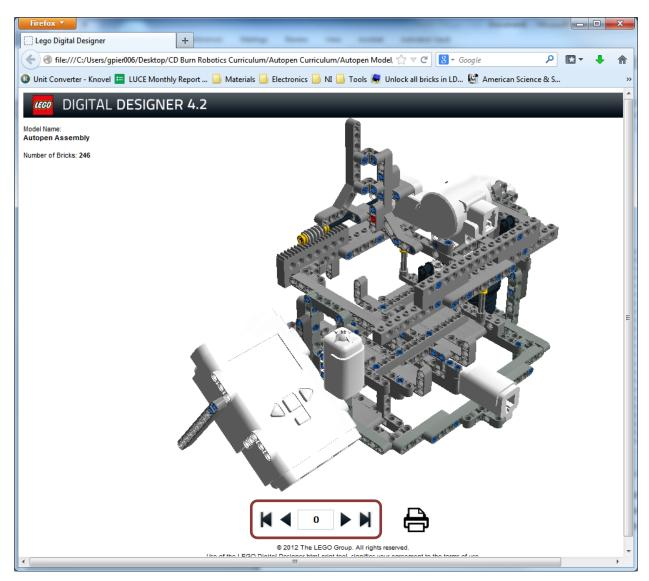
Use the arrows found at the bottom of the screen to advance or go back in the build process. Note the build instructions indicate the parts needed for that portion of the build as well as what your part should look like once assembled.
