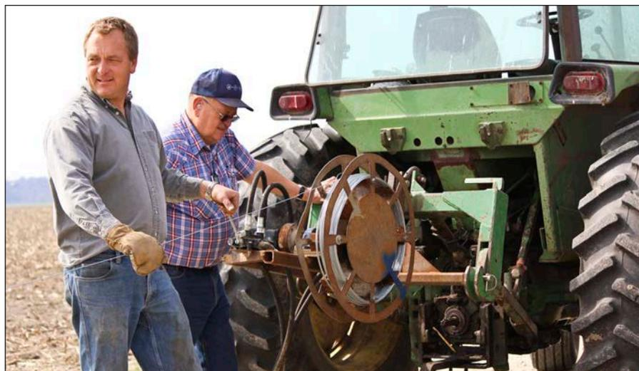
**ROLL IT UP:** Trying to keep down the cost of the fencing system, Kelly Forck (left) explains to his dad, Pee Wee, just how the operation rolls up wire. Kelly designed the wire roller to be portable, using the power from the tractor to roll up hundreds of feet of electric fence.
